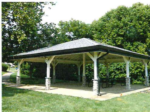
There is a pavillion adjacent to the playground. The pavillion is on a concrete slab that is 34' x 34'. There are nine wood support poles 5" x 5" x 8' (h). The roof is constructed of wood with asphalt shingles and guttering on four sides with two downspouts. There is an electric light on the ceiling. Amenities include two metal picnic tables 2' 6" x 8'; two metal trash cans; 1 charcoal grill; and 1 metal bench.
